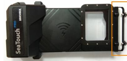
EN Please check the top cover and keep it open when you take the housing on board or put it into your luggage. The lower air pressure on plane would lead to the housing inflated if the cover is sealed, which could cause serious damage to the touch membrane of the housing.
